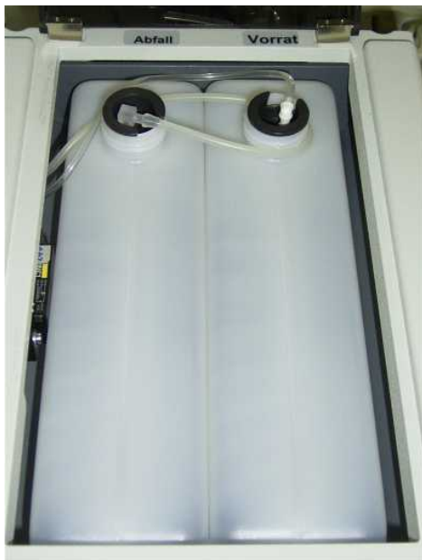
fig. 6.5 view of supply and waste container
